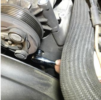
Remove the 4 bolts holding the AC compressor but leave the compressor in place. Then remove the front accessory bracket bolt as shown.
