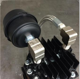
**Standard compressors:** Verify the O-rings are present in the bottom of each of the head fittings and install on the compressor. The filter/silencer will go on the port labeled "Suction". **SLM compressors**: Install the filter/silencer into the suction port side, labeled with an "S". Make sure to hold the 90 fitting with a wrench so as not to break the fitting or compressor head while tightening.
