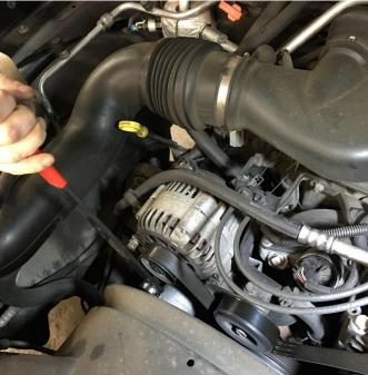
Start by making a witness mark across the idler pulley arm to indicate the factory belt tension. Next, rotate the idler pulley to remove the belt. Then remove the factory alternator bolt. You may wish to remove the upper fan shroud at this time to make the installation easier, but it is not required.
