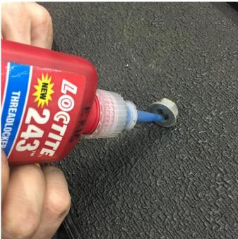
Remove the factory power steering bracket as shown and apply medium strength thread locker to the nut (such as Loctite 243).
