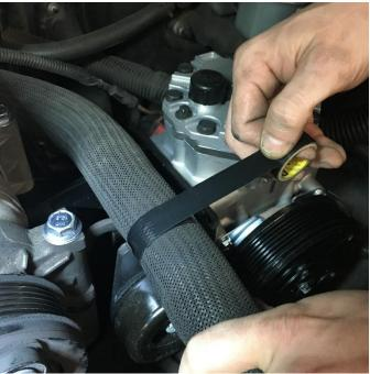
Four 3/8 bolts and lock washers are provided for mounting the compressor to the bracket. They should be tight but be careful not to strip the aluminum compressor body. After the compressor is mounted, it is advised to wrap a few runs of electrical tape over the area where the upper radiator hose will sit (not applicable to all models). Some models carry a throttle cable bracket, which may be mounted back through the EDC bracket and into the original threaded hole.
