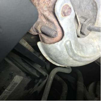
Insert the supplied compressor spacer and start the M10x1.5x100mm bolts on that side, but do not tighten. Start installing the compressor bracket by slipping the slotted opening over the power steering stud as shown.
