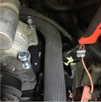
Start the 3/8-16 x 5.0 bolt and washer through the bracket and into the head, but do not tighten. Then start the remaining M10x1.5x100mm through the AC compressor and the bracket. You may need to use an adjustable wrench to apply pressure in or out until the bolts register into their threads. After all bolts are started, confirm that the slotted foot of the bracket is seated on the power steering stud and tighten all bolts including the power steering stud nut.
